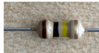
(b) 100 kΩ with a ±10% tolerance
