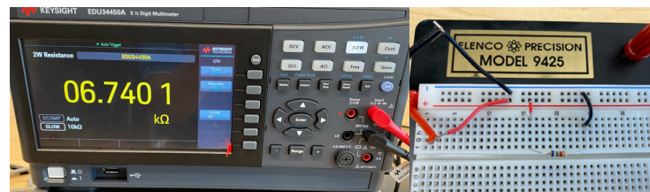
Fig. 6. Ohm's Law verification circuit on a breadboard
