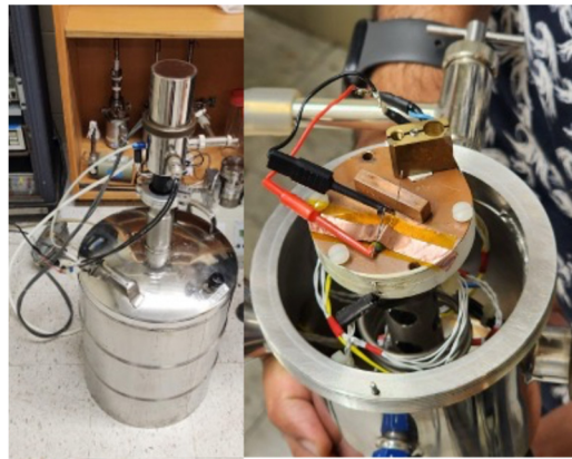
Fig. 18. Cryocooler setup and electrical wiring configuration for the resistivity experiment, showing measurements for both a normal (non-superconducting) resistor and a superconducting YBCO sample.
